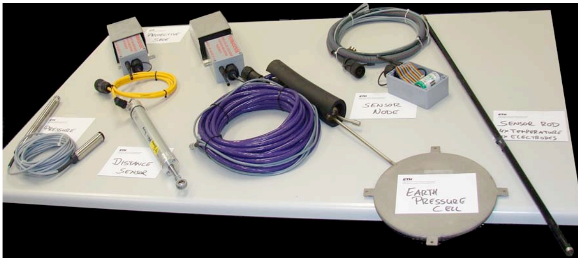
Figure 4: Overview of applied sensors: Water / air pressure sensor (WP), crackmeter (CR), earth pressure cell (EP), and sensorrod (SR); (other sensors (TC/TM/SP) not shown).
