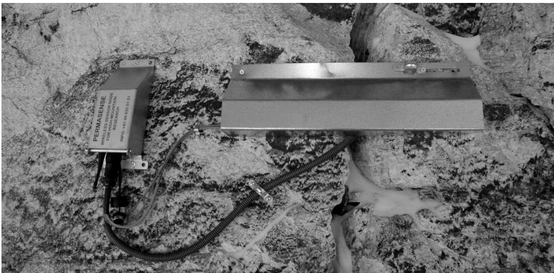
Figure 5: Sensor node consisting of the network node inside of the protective shoe (left), a crack-meter below the shield (right) and a thermistor chain inside the cleft (dark cable).
